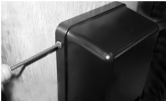
FIG. 16: SECURE TOP OF INSIDE HOUSING
