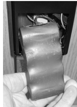
FIG. 18: INSERT BATTERY PACK INTO HOUSING
