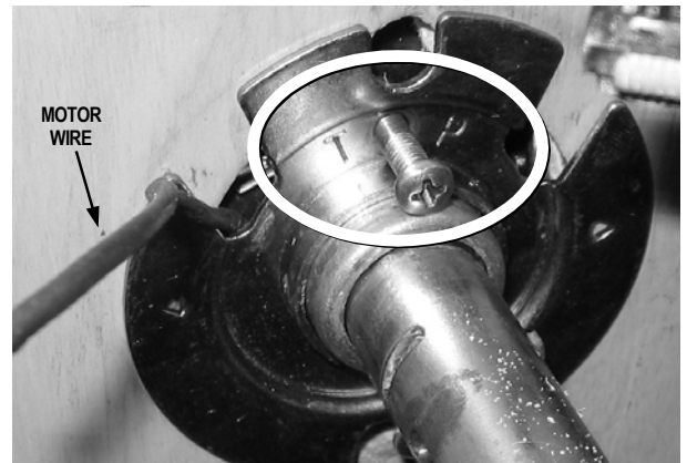
FIG. 12: INSIDE ROSE PLATE INSTALLATION
